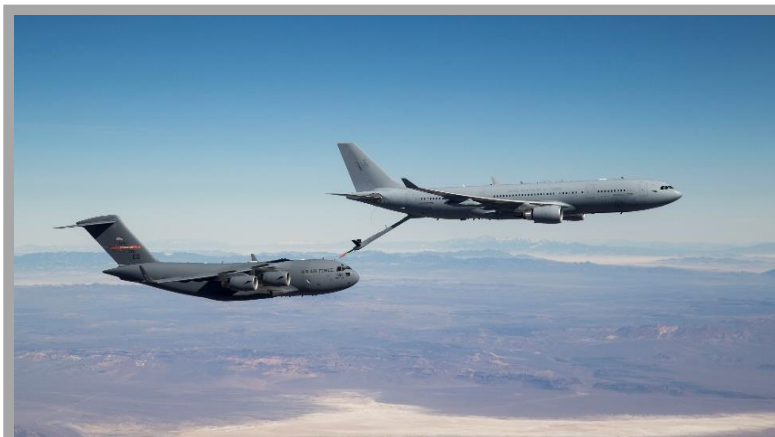
A Royal Australian Air Force KC-30 tanker connects with a US Air Force C-17 as part of the Coalition Tanker Aerial Refueling Certification Effort. (US Air Force Photo)
